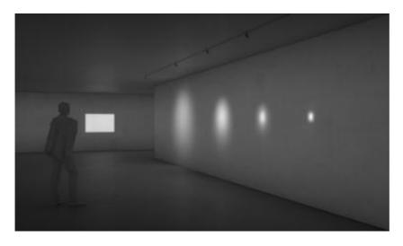
Fig. 3: Visualization picture framing SUPERSYSTEM and 40, 24, 16 and 8 degrees reflector.
