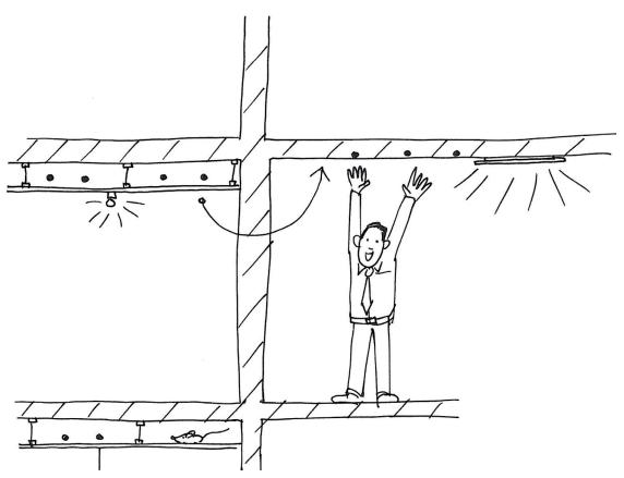
B5 I Lower buildings thanks to omission of suspended ceilings and false floors, and consequently lower construction costs.
