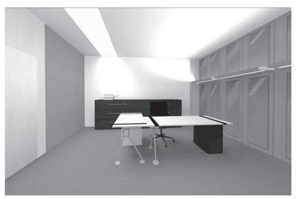
B3 I Room lighting concept: Two components ensure appropriate ambient illuminance across the entire office area: a luminaire integrated into the façade, which radiates light indirectly via the ceiling and into the direction from which daylight is entering, and a flat wide-area luminaire ("artificial skylight") with direct distribution located in the depth of the room.
